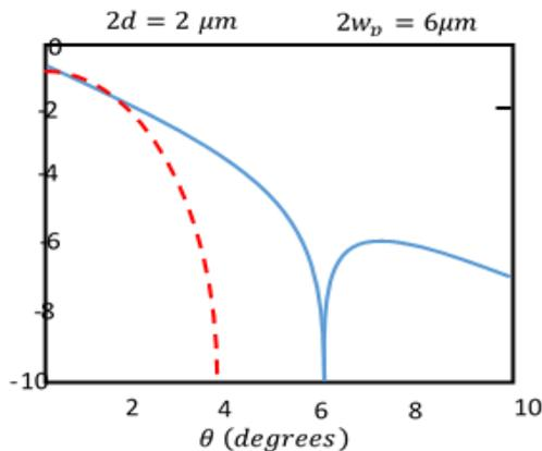
**Fig. 3.** Logarithm of reflection coefficient as a function of mirror tilt angle for mode power full width  $6\mu m$  and slab full width  $2\mu m$ .
