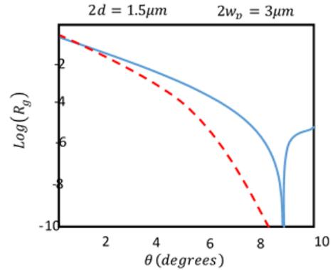
**Fig. 2.** Logarithm of reflection coefficient as a function of mirror tilt angle for mode power full width  $3\mu\text{m}$  and slab full width  $1.5\mu\text{m}$ .
