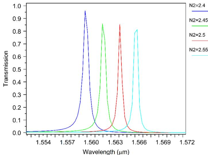
**Fig.5.** The output spectra of the filter for different values of N.
