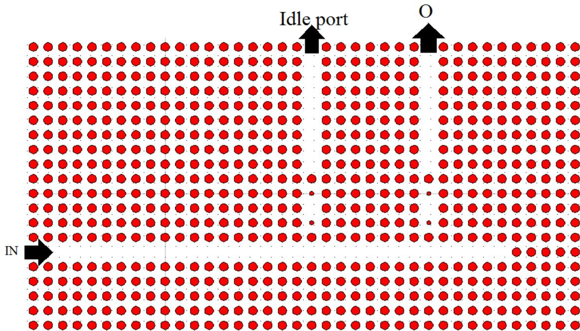
**Fig.6.** The optical FSK demodulator.
