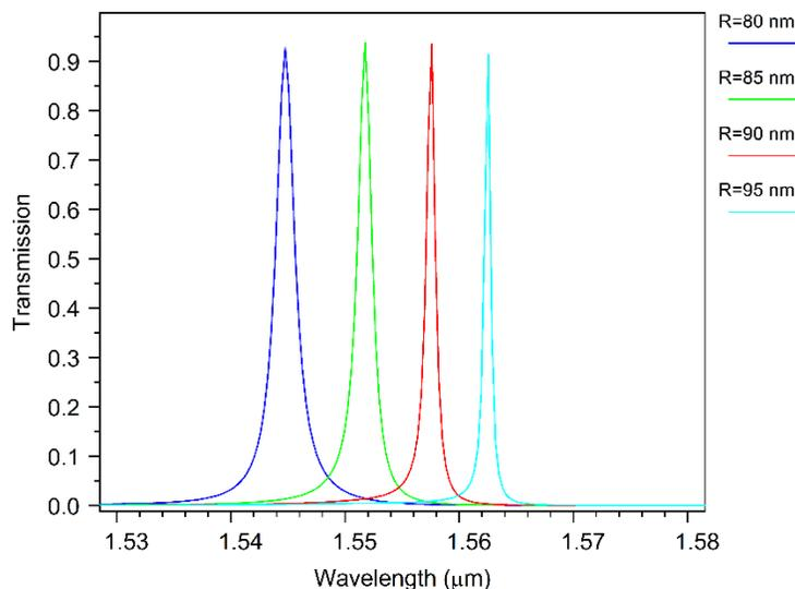
**Fig.4.** Output spectra of the filter for different values of R.
