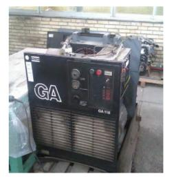
Fig.5. GA111 compressor of Atlas Copco Company
