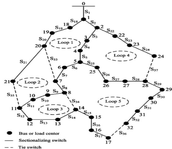
Fig. 4. The 33-bus sample system with loop numbers
