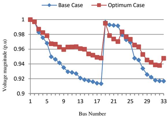
**Fig. 6.** Comparison of voltage magnitude of 33-bus system.
