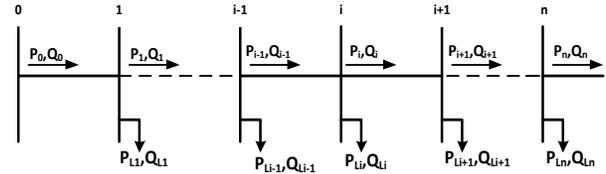
**Fig. 1.** Single-line diagram of a main feeder
