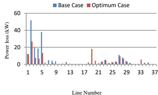
**Fig. 7.** Comparison of power loss at each line of 33-bus system.
