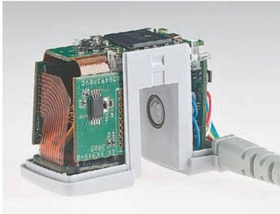
Fig.10. The Internal Circuitry Capnograph Sensor (sensor CO_2 )
