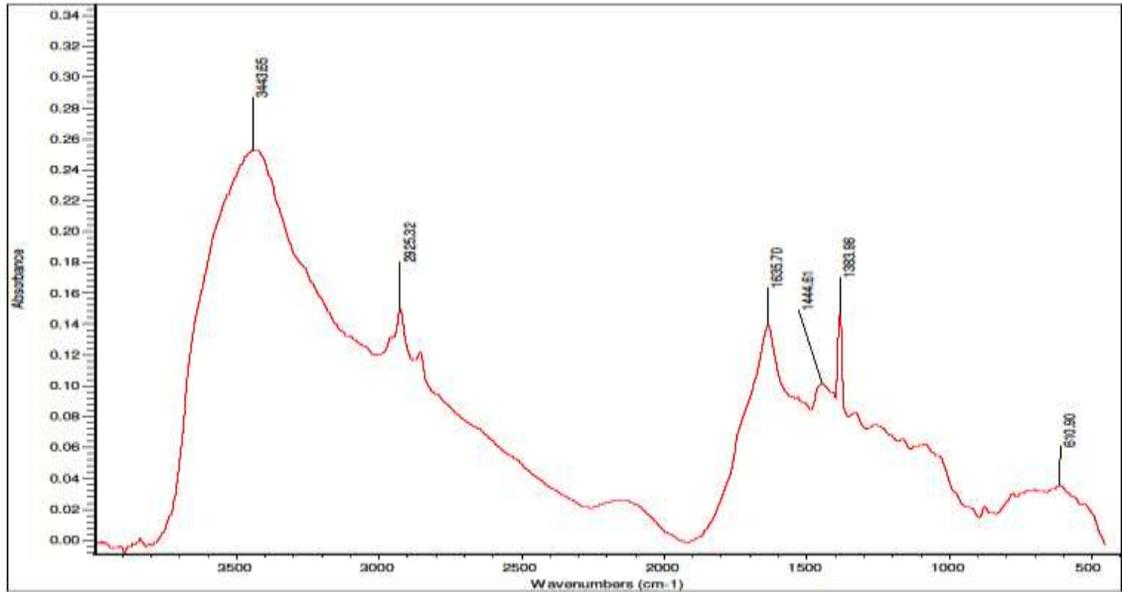
**Figure. 2.** FT-IR of gelatin scaffold (27 wt.% in 50% acetic acid ,20% water) mixed at 50:50 (v/v) ratio].
