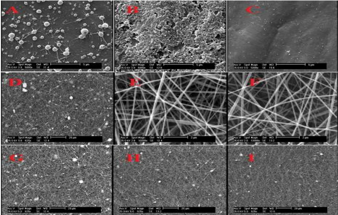
**Figure 1:** A: Voltage :10 kV,TCD:10 cm-B:Voltage:10 kV,TCD:15cm-C:Voltage:10 kV,TCD:20 cm D:Voltage:12 kV ,TCD:10 cm-E:Voltage :12kV,TCD:15cm-F:Voltage:12 kV,TCD:20 cm G:Voltage:15 kV,TCD:10 cm-H:Voltage15 kV,TCD:15 cm-I:Voltage:15 kV,TCD:20 cm.
