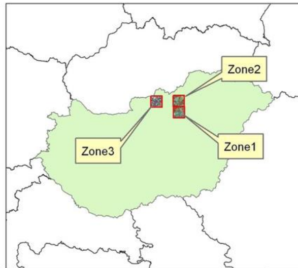
Figure 1. Location of the test zones in Hungary. Each test zone is a 24\text{ km} \times 24\text{ km} square region. For each zone, a 5-band (blue, green, red, red-edge and near-infrared) 4800 \times 4800 pixel Rapid Eye image is used for LPIS assessment with the proposed method.
