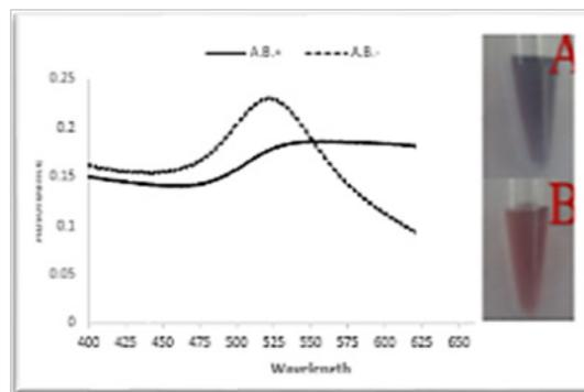
Fig. 12. Changes of wavelength and colorimetric resulting from connection of multiplex probes to target sequences in a positive control sample (A) compared to the negative control (B)
