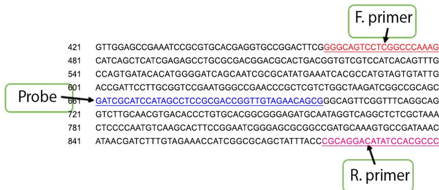
Fig. 2.Part of the *hpt* gene, and position of designed Primers and probe
