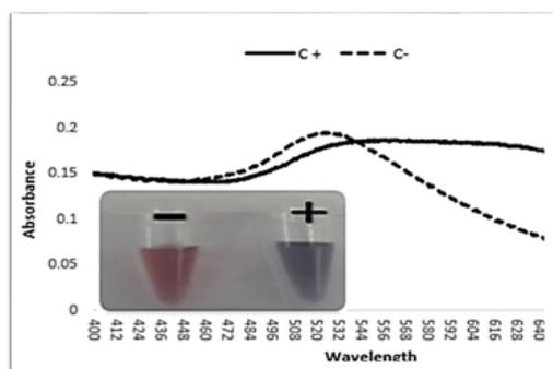
Fig. 11. colorimetric and wavelength changes resulting from single probes for *hpt* gene binding to target sequences in a positive control sample (+) in comparison with the negative control (-)
