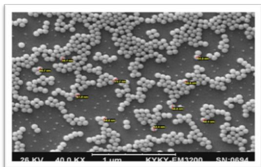
Fig. 7. Image of gold nanoparticles synthesized by trisodium citrate taken by TEM
