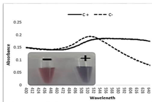
Fig. 10. Changes in wavelength and colorimetric resulting from single-bind probe for GUS gene to target sequence in positive control sample (+) compared to the negative control (-)
