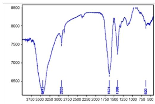
Fig. 8. FT-IR spectrum of synthesized gold nanoparticles
