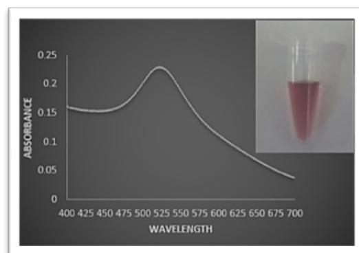
Fig. 9. Absorption spectrum of gold nanoparticles, as shown in the picture, the maximum absorption of gold nanoparticles occurred at the wavelength of 525 nm
