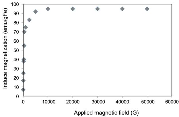
Fig. 3: CMn-Fe nps magnetization curve measured by SQUID exhibiting magnetic saturation
