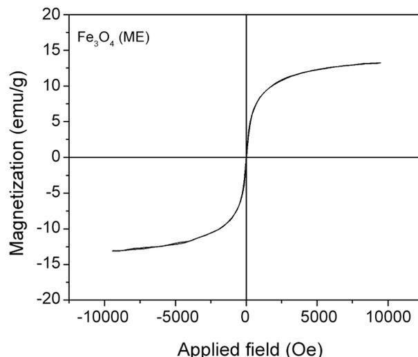
Fig. 3: Magnetic hysteresis curve of samples produced by mercaptoethanol inhibitor  $\text{Fe}_3\text{O}_4$  (ME).
