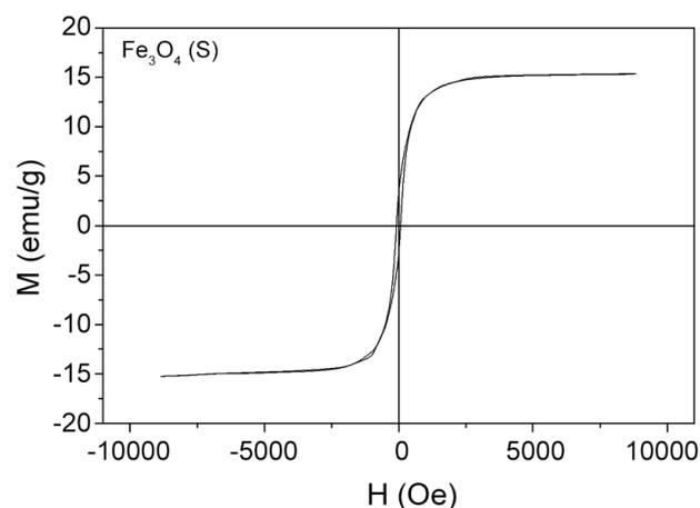
Fig. 4: Magnetic hysteresis curve of  $\text{Fe}_3\text{O}_4$  samples produced by starch as inhibitor.
