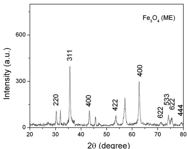
Fig. 1: XRD pattern of  $\text{Fe}_3\text{O}_4$  samples produced by mercaptoethanol as inhibitor.
