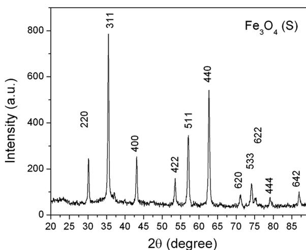
Fig. 2: XRD pattern of  $\text{Fe}_3\text{O}_4$  samples produced by starch as inhibitor.
