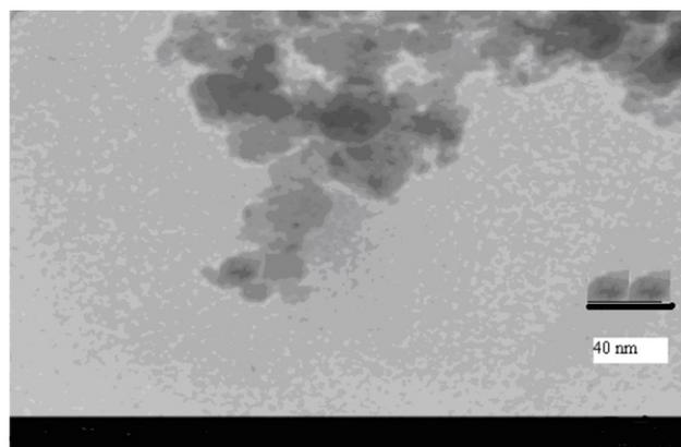
Fig. 5: TEM micrograph of Fe<sub>3</sub>O<sub>4</sub> samples produced by starch as inhibitor.
