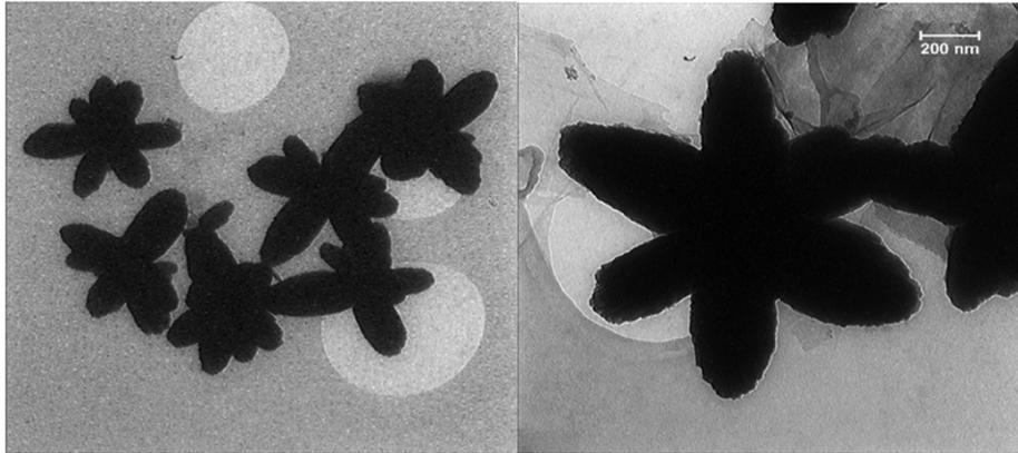
Fig. 2. Transmission Electron Microscope of ZnO:Fe nanoflower.
