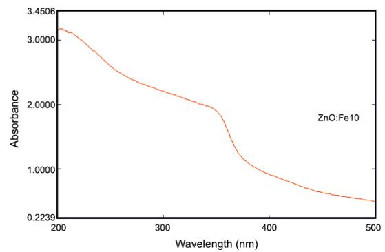
Fig. 3. (a) UV-Vis absorption spectrum of ZnO, (b) UV-Vis absorption spectrum of ZnO:Fe.
