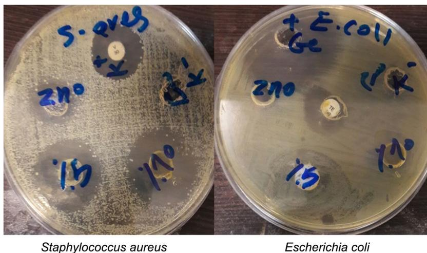
Fig. 4. Antibacterial activity of ZnO, ZnO:Fe %5 and ZnO:Fe %10 nanoparticles Staphylococcus aureus and Escherichia coli.
