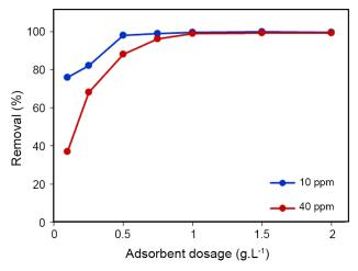
Fig. 6. Effect of organomodified nanoclay dosage on dye adsorption
