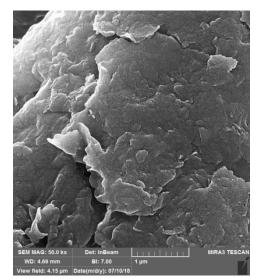
Fig. 4. SEM image of Organomodified nanoclay.
