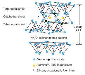
Fig. 1. Layered silicate structure [19]
