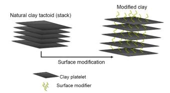
Fig. 2. Nanoclay structure modification scheme
