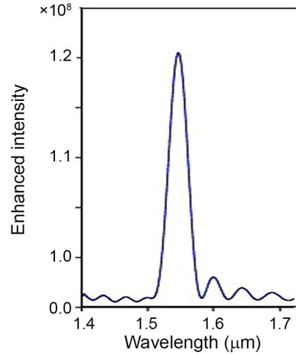
Fig. 3. Optical Field Intensity improvement at resonance wavelength (InGaAsP quantum wells nanocavity).
