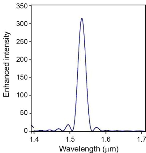
Fig. 2. Optical Field Intensity improvement at resonance wavelength (InP nanocavity).
