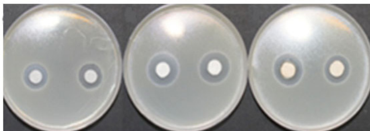
Fig. 12. Antimicrobial activity of s-PBI/cellulose/silica hybrid nanocomposites with (a) B. cereus (+) and (b) E. coli (-) for 24 h incubation at 37°C
