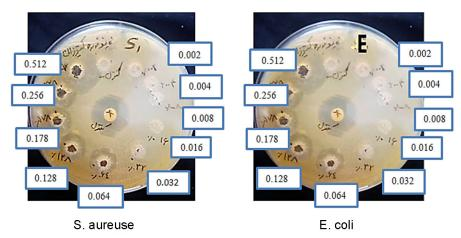
Fig. 1. Zone of inhibition for different concentration (g/ml) in standard E.coli & S.aureus against chitosan nanoparticle
