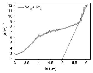
Fig. 1. The corresponding linear portion of the plots of  $(\alpha h \vartheta)^{1/2}$  against h $\vartheta$
