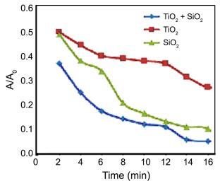
Fig. 2. Decolorization of MB dye of  $\rm{SiO}_2, \rm{TiO}_2$  and  $\rm{SiO}_2/\rm{TiO}_2$  nanomposite materials
