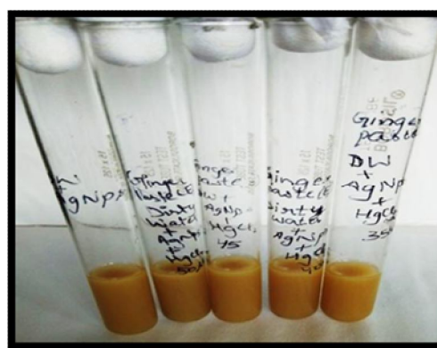
Fig. 14. Shows the detection of metal ion in the synthesized silver nanoparticles from Zingiber officinale paste in 70% ethanol and C.W at 630 nm.
