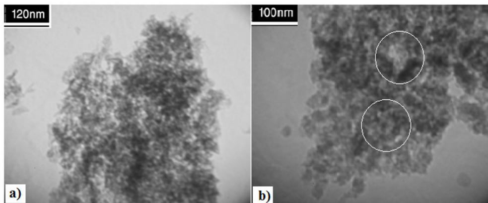
Fig. 5a,b. TEM image of: a) nHAp synthesized in 2.8 g collagen matrix before and (b) after silica coating.
