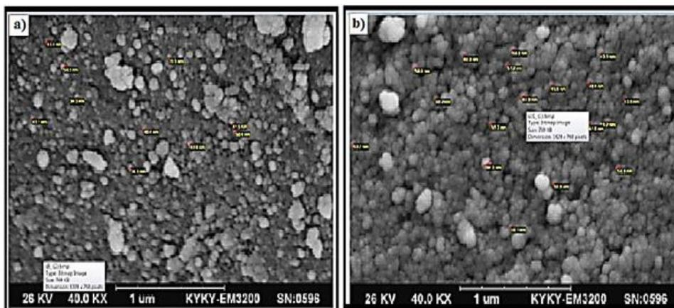
Fig. 3. SEM image of nHA synthesized in 2.8 g collagen: a) before and b) after 72 hrs immersion in SBF solution.
