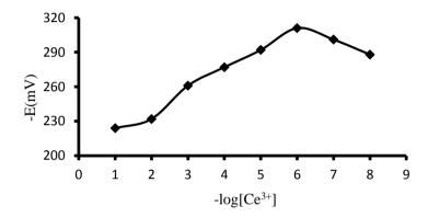
Figure 2. Calibration curve of the Ce<sup>3+</sup> selective sensor based on kryptofix22DD.
