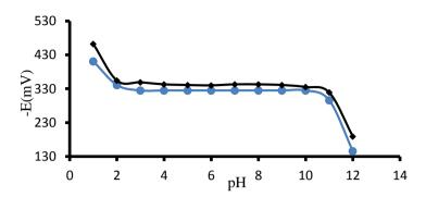
**Figure 5.** Effect of the pH of test solutions on potential response of the  $Ce^{3+}$  selective sensor ( $\bullet$  1.0×10<sup>-3</sup> M,  $\bullet$  1.0×10<sup>-4</sup>M).
