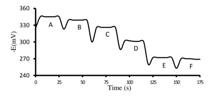
**Figure 4.** Dynamic response time of the  $Ce^{3+}$  selective sensor for step changes in the concentration of  $Ce^{3+}$ : (A)  $1.0\times10^{-6}$  M, (B)  $1.0\times10^{-5}$  M, (C)  $1.0\times10^{-4}$  M, (D)  $1.0\times10^{-3}$  M, (E)  $1.0\times10^{-2}$  M, (F)  $1.0\times10^{-1}$  M.
