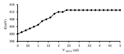
**Figure 6.** Potentiometric titration curve for 25 ml  $1.0 \times 10^{-3}$  M of Ce<sup>3+</sup> solution with  $1.0 \times 10^{-2}$  M of EDTA.
