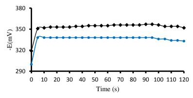
**Figure 3.** Static response time curves of the Ce<sup>3+</sup> selective sensor ( $\bullet$  1.0×10<sup>-3</sup> M,  $\bullet$  1.0×10<sup>-4</sup> M).
