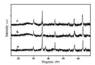
Fig. 2. XRD pattern of (a) MNPs, (b) Si-MNPs and (c) Mn (salophen)-imid-Si@Si-MNPs
