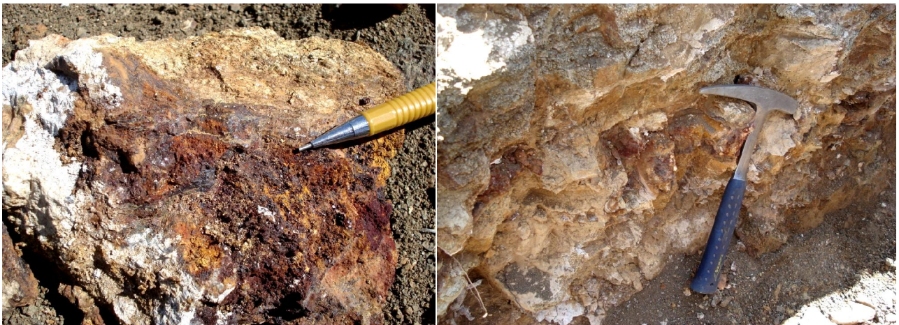
Fig. 5. Right) Argillic and sericitic alteration in the gabbro diorite contact; Left) Fe- oxide impregnation (goethite) together with argillic alteration.
