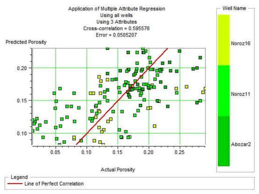
Fig. 5. A cross plot showing the relationships between actual and predicted porosity.
