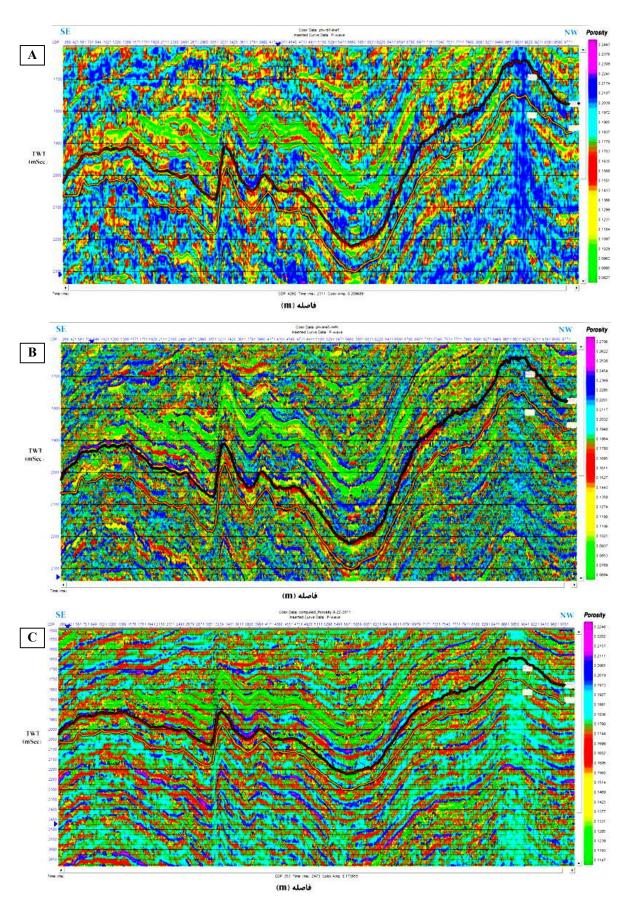
Fig. 7. Predicted porosity for the Bourgan reservoir across the Nowrooz oil field: (A) RBFN, (B) MLFN, (C) PNN.
