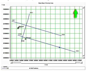
Fig. 2. A 2D Map showing the location of wells and 2D seismic sections across the Burgan reservoir.
