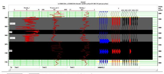
Snap to: Snap Peak/Trough 💌 Wavelet wave1 💌 Current Corr: 0.810 Max Corr: 0.810 at time shift: 0 ms Apply Shift Parameters ... Fig. 4. A sample of well to seismic tie at well A-2.
