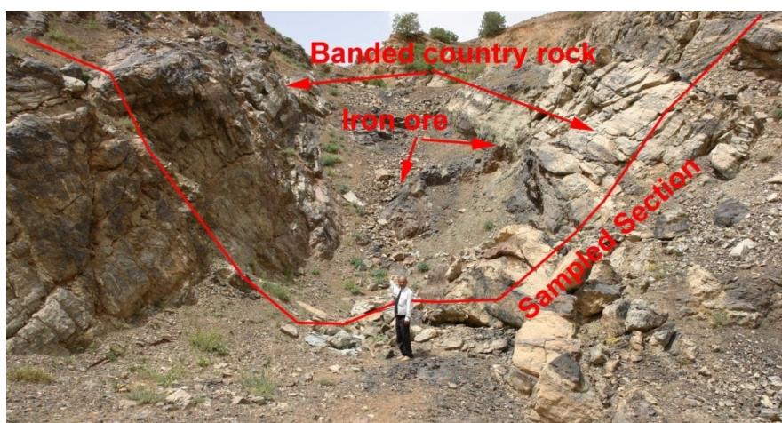
Fig. 4. Upper Quarry of the Asnawa iron ore (S3 samples section) shows partial and veinal replacement of country rocks (banded hornfels) by iron
