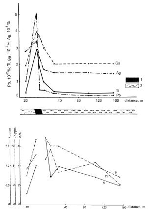
Fig. 2. Dependence of components content in host rocks with reference to distances away from the ore (Filizchai deposit) Legend: 1 – ore body; 2 – host rock
