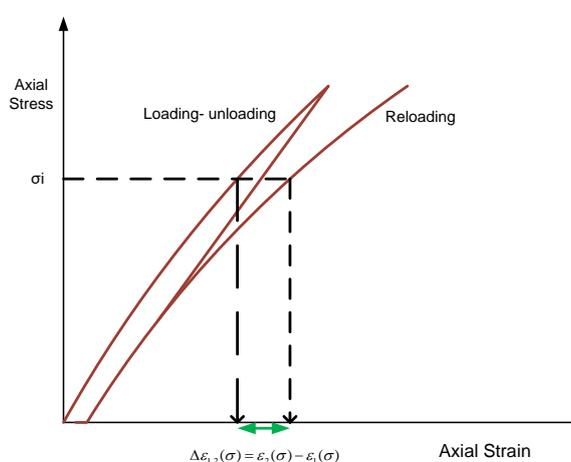
Fig 1. Fundamental concept differential strain used in the DRA
