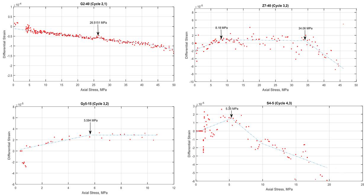
Fig 5. Variation of strain difference versus axial stress, (a) granite (b) zeolite (c) gypsum (d) sandstone
