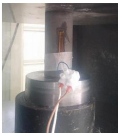
Fig 3. a) Prepared core samples from rock blocks of sandstone for DRA testing, b) sample under DRA testing
