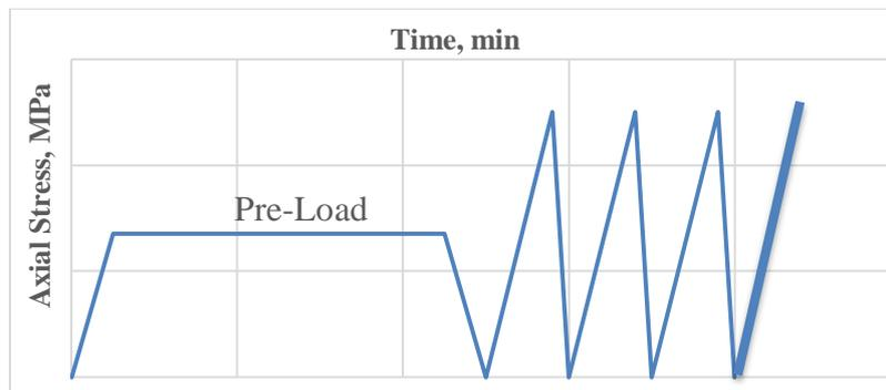
Fig 4. Uniaxial loading-unloading path for DRA tests
