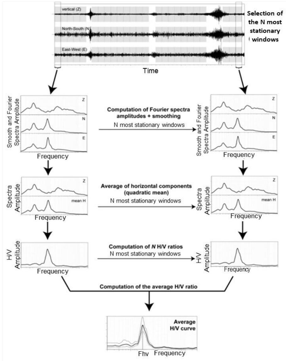
Fig 2. The flowchart shows the computation steps of the H/V ratio (Fergany and Omar 2017).
