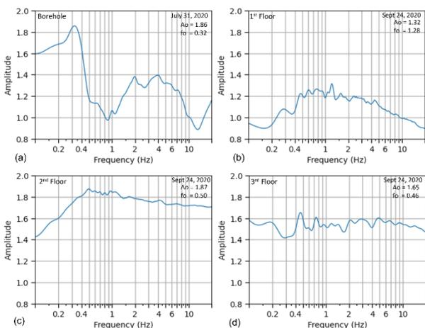
Fig 7. The horizontal to vertical spectral ratio curve of microtremor data processing results on the 1<sup>st</sup>, 2<sup>nd</sup>, and 3<sup>rd</sup> floors
