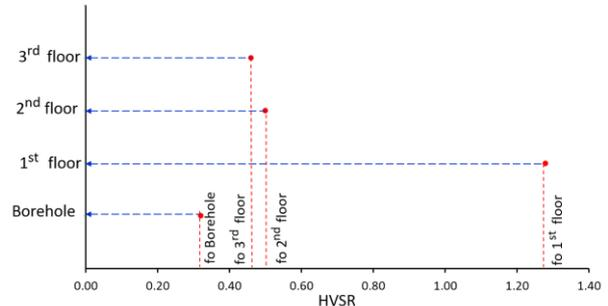
Fig 8. Graph of the relationship between the location of the microtremor measurement in the BMKG Region III Denpasar building with  $f_0$  HVSR value.
