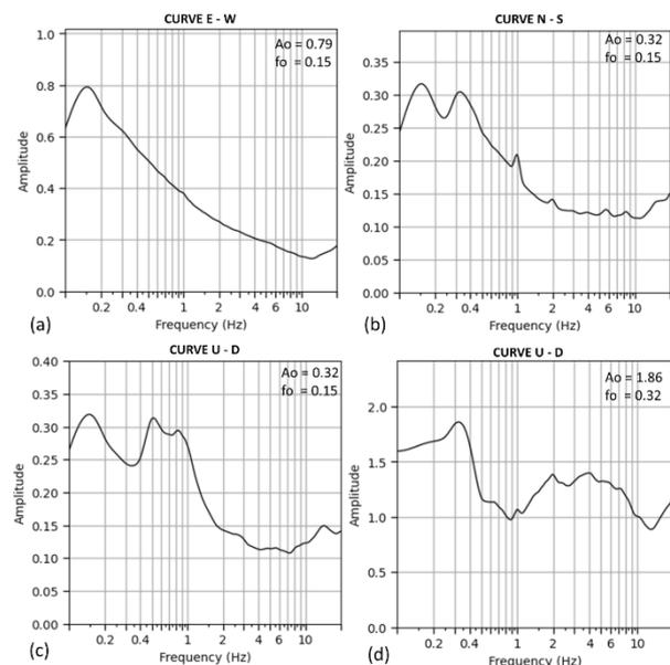
Fig 5. The results of processing the fast Fourier transform microtremor data to obtain the natural frequency value of the waves and the HVSR curve to obtain the natural frequency of the soil for the data on July 31, 2020. (a) The natural frequency
