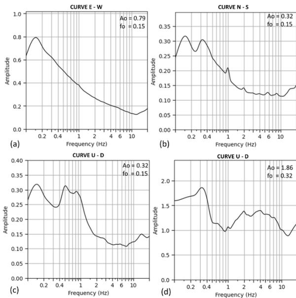
Fig 6. The results of processing the fast Fourier transform microtremor data to obtain the natural frequency value of the waves and the HVSR curve to obtain the natural frequency of the soil for the data on July 31, 2020. (a) The natural frequency curve of the E-W component microtremor wave; (b) The natural frequency curve of the N-S component microtremor wave; (c) The natural frequency curve of the Z (U-D) component microtremor wave; and (d) The HVSR curve of the soil ( $f_0$  HVSR).
