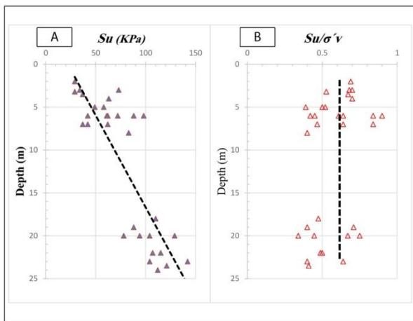
Fig. 7. Undrained shear strength ( $S_u$ ) from unconfined compression test (UC): (A)  $S_u$  versus depth and (B) Normalized values of undrained shear strength relative to effective stress versus depth
