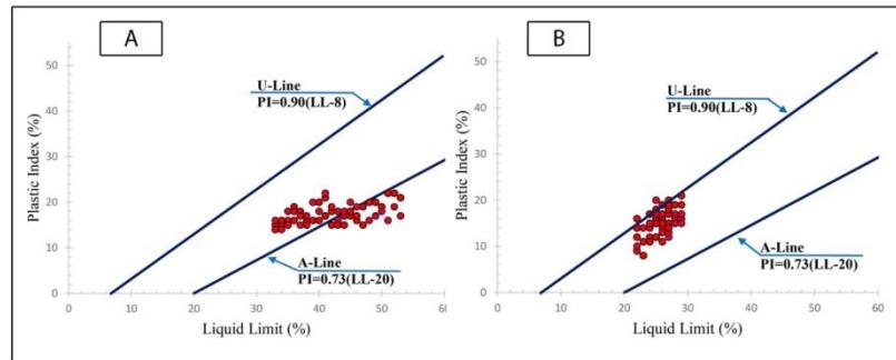
Fig 5. Correlations between plasticity index and liquid limit of fine-grained soil in Gorgan: (A) low-plasticity clay related to the UCU engineering layer and (B) low-plasticity clay related to the LCU engineering layer
