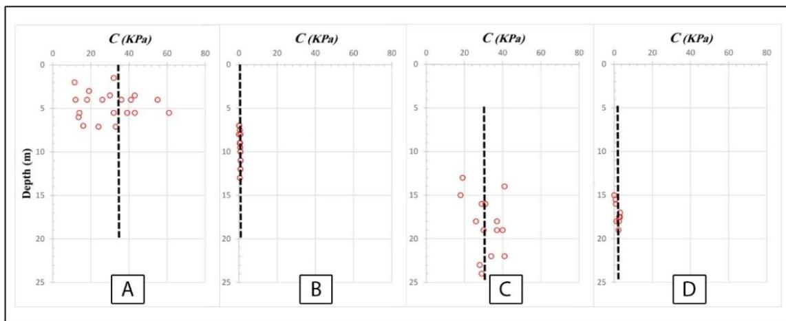
Fig. 9. Variation of cohesion values obtained from direct shear test versus depth: (A) the data for the UCU, (B) the data for the MGU, (C) the data for the LCU, and (D) data relating to the SU
