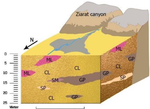
Fig 4. The three-dimensional (3D) geological model of subsurface soil in Gorgan city
