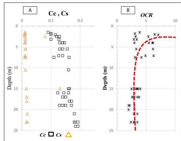
Fig 6. Compressibility of fine-grained soil in the Gorgan: (A) Compression index ( $C_c$ ) and swelling index ( $C_s$ ) versus depth and (B) over-consolidation ratio (OCR) versus depth
