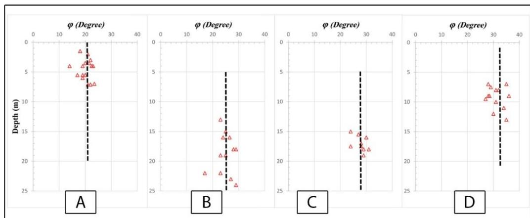
Fig. 8. Variation of internal friction angle obtained from direct shear test versus depth: (A) the data for the UCU, (B) the data for the MGU, (C) the data for the LCU, and (D) data relating to the SU
