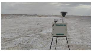
Fig 2. Ambient point dust monitor near drilling activity in limestone benches
