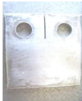
Fig.8 Marking and crack creating on specimens.
