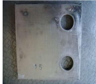
Fig.7 Marking and drilling of specimens.
