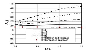
**Fig.2** values of  $\lambda_j$  for different values of the angle of inclination  $(\theta_i)$  and dimensionless parameter  $(h/R_b)$ .
