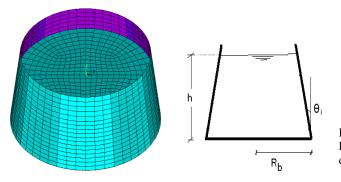
**Fig.5** Finite element modeling and geometric coordinate system of tank.
