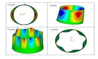
**Fig.3** Circumferential mode shapes for the *1st* axial mode.
