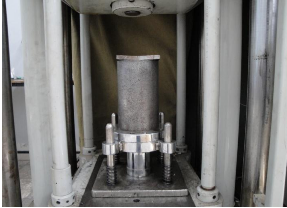
Fig.3 A schematic view of the die and hydraulic press.
