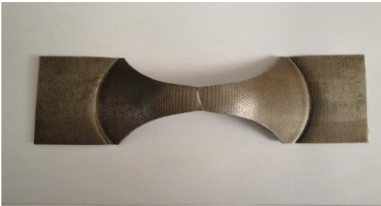
Fig.4 Sample stamped specimens used for FLD determination with fracture after testing.
