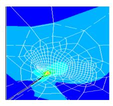
Fig. 5 Discretization and distribution of stresses for  $\alpha = 45^{\circ}$ .
