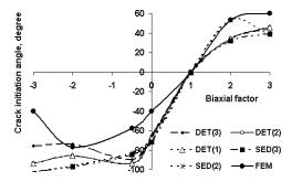
Fig. 8 Comparison of crack initiation angle predicted by finite element method (FEM) with other theoretical predictions under different biaxial load for crack angle,  $\alpha = 45^{\circ}$ .
