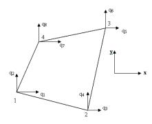
**Fig. 4** Four node quadrilateral element, *q*: element displacements.
