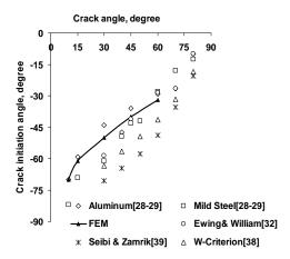
**Fig. 6**Comparison of crack initiation angle predicted by Finite Element Method (FEM) with experimental results.
