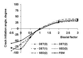
**Fig. 9** Comparison of crack initiation angle predicted by finite element method (FEM) with other theoretical predictions under different biaxial load for crack angle,  $\alpha = 30^{\circ}$ .
