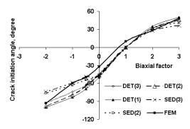
Fig. 7 Comparison of crack initiation angle predicted by Finite element method (FEM) with other theoretical predictions under different biaxial load for crack angle,  $\alpha = 60^{\circ}$ .
