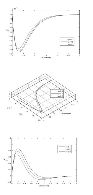
Fig. 13 Stress distribution  $\sigma_{xy}$  with variation of distance under GL theory.
