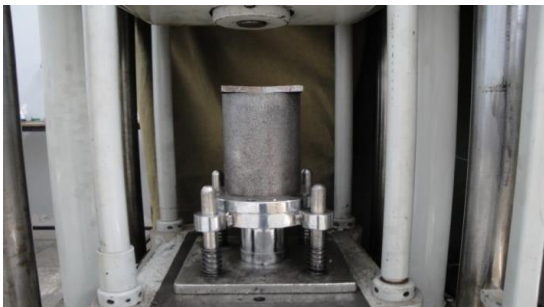
Fig.3 A schematic view of the die and the hydraulic press.
