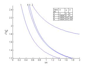
Fig. 7 Effect of different combinations of the initial stresses  $(\xi', \xi)$  on the propagation of Love waves for  $\mu_0 / L = 2.50$ , b/k=0.4, a/k=1,  $\gamma = 4$ , and  $\beta_a / c_{as} = 0.7$ .
