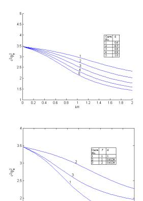
Fig. 2 Velocity dispersion curves of Love waves in a porous layer for various porosity in terms of parameter *d* and for  $\mu_0 / L = 2.50$ ,  $\gamma = 1$ , b/k=0.4, a/k=1,  $\xi = \xi' = 0$ , and  $\beta_a / c_{ex} = 0.7$ .
