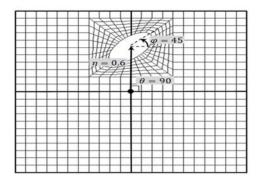
**Fig. 7** Plate with cutout in an arbitrary position and orientation.
