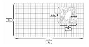
Fig. 2 Mesh structure of the plate.
