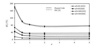
Fig. 4 Comparison of critical thermal buckling temperature versus n for a square plate without hole with Ref. [4].
