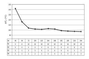
Fig. 3 Convergence investigation of a rectangular plate of aspect ratio a/b=2.5 with a centrally located elliptic cutout and (CC) BCs.
