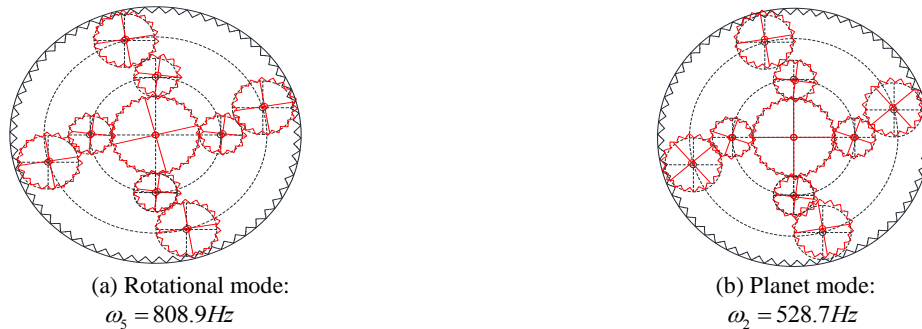
Fig.13 Types of vibration modes of the ASS with four planet trains (planet 1: 0, 80, 180 and 260 degree and planet 2: 40, 120, 220 and 300 degree).
