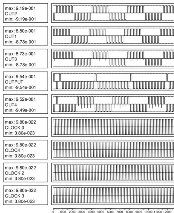
Fig. 10. The results of circuit simulation with QCADesigner.
