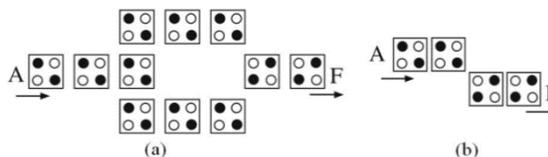
**Fig. 4. Inverter gates**
