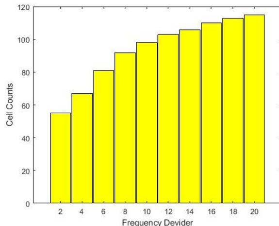
Fig. 13. The cell counts of the circuits according to the output frequency.
