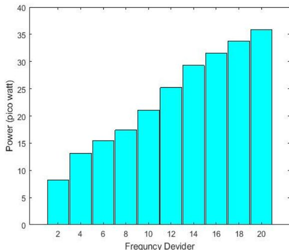
Fig. 12. The power consumption of the circuits according to the output frequency.
