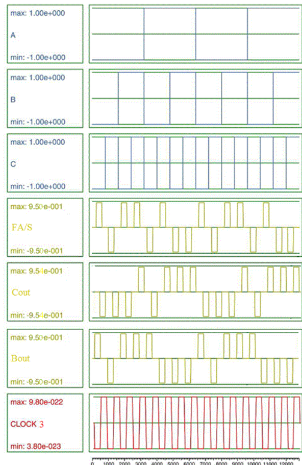
Fig. 32. Simulation result of the proposed Full Adder/Subtractor circuit in Fig. 26-b.
