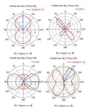
Fig. 5. Radiation pattern of Vivaldi antenna at different frequencies 3, 6.8571, 9.428, 12 GHz respectively.
