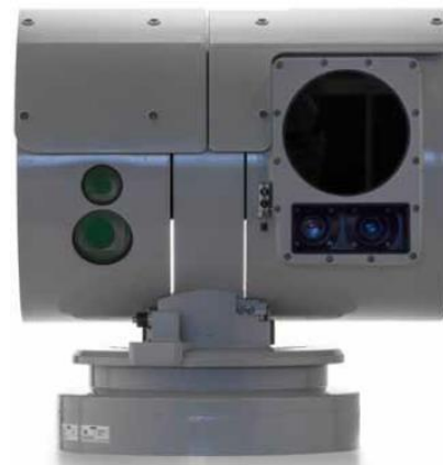
Fig. 6. Electro-Optical Fire Control Director (SAAB Company).
