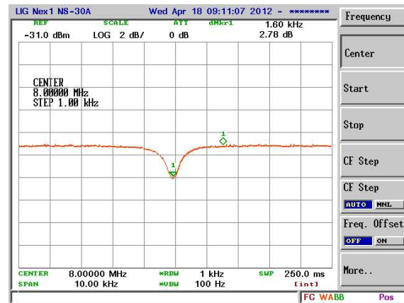
Fig. 5.b. Frequency response of single crystal resonator circuit in Spectrum Analyzer ( BW_{3dB}=0.7K loss=3dB)
