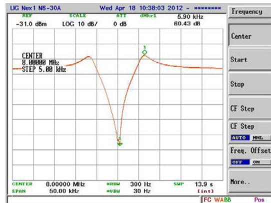
Fig. 7.b. A crystal filter response in the spectrum analyzer ( BW_{3dB} = 10K loss = 60dB = 10K )
