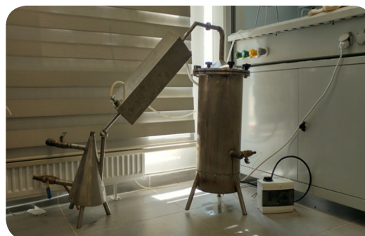
Fig. 2. The distillation apparatus was designed by Ayhan AKPEK for boiling fruit pulps (pictured by Mehmet Ali DEMİRÇİ at Çankırı Karatekin University).
