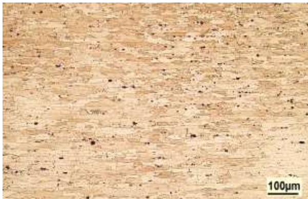
Fig. 4 Optical micrograph of the AA7075 base metal.
