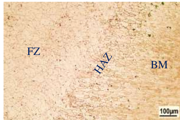
Fig. 9 Optical micrograph of different zones of artificially aged joint.
