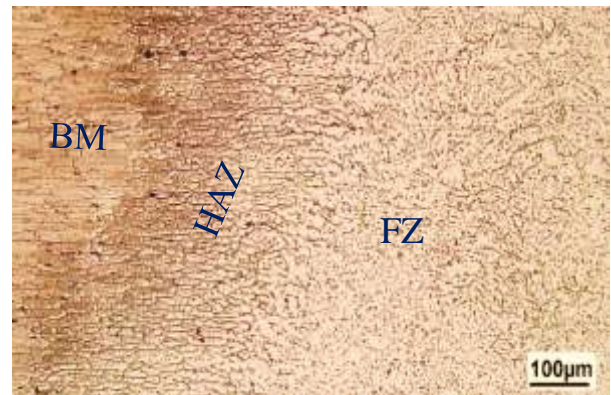
Fig. 6 Optical micrograph of HAZ and FZ of the WB.
