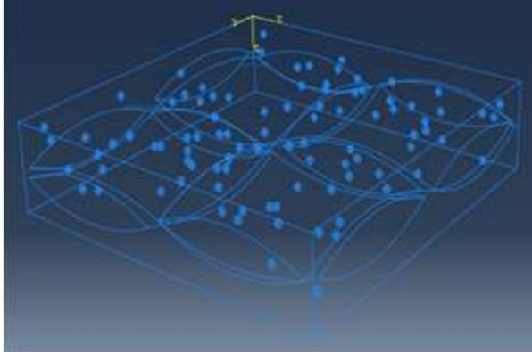
Fig. 3 Composite unit cell along with nanoparticles.
