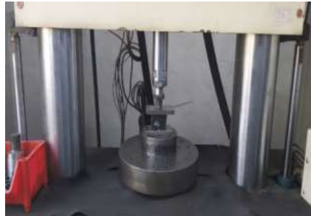
Fig. 7 Harmonic dynamics testing device of Iran spare parts manufacturing company.
