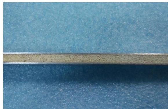
**Fig. 3** Standard specimens for flexural test.
