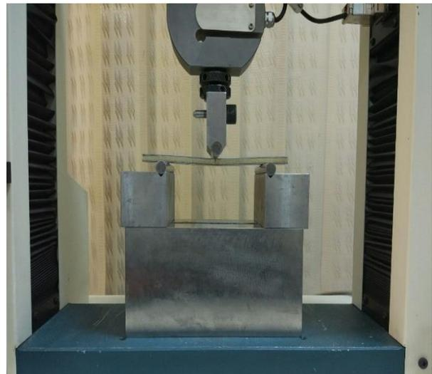
**Fig. 5** Flexural test machine with the three-point bending fixture and the specimen.
