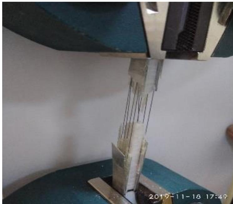
Fig. 6 Specimen after rupture in tensile test.
