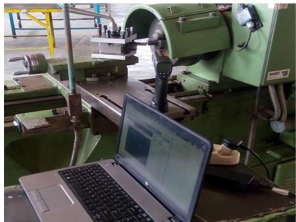
Fig. 2 Recording temperature during machining.
