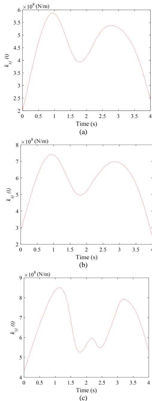
Fig. 7 Mesh stiffness variations of sun- $j^{\text{th}}$  planet with: (a)  $\alpha_{sj} = 20^\circ$ , (b)  $\alpha_{sj} = 25^\circ$  and (c)  $\alpha_{sj} = 30^\circ$ .
