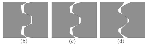
Fig. 5 Model of gear meshes by: (a) finite element with (b) 20° (c) 25° and (d) 30° pressure angle of gears.
