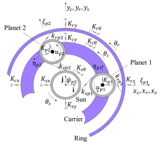
Fig. 1 Lumped parameter model of the planetary gear and system coordinates.
