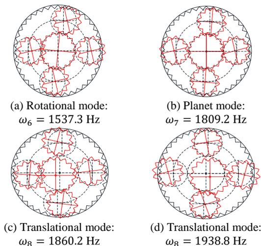
Fig. 12 Types of vibration modes of the ASS with four planets (0, 80, 180 and 260 degrees).
