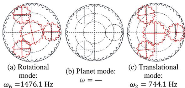
Fig. 11 Types of vibration modes of the SS with three planets (0, 120 and 240 degrees).
