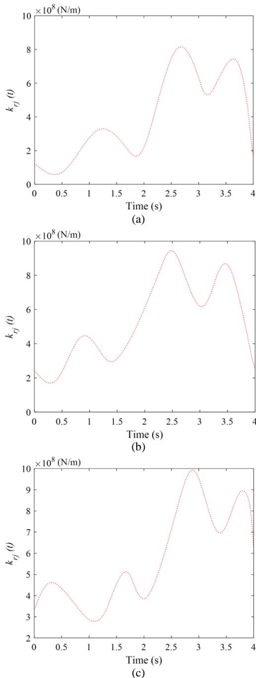
Fig. 6 Mesh stiffness variations of ring- $j^{\text{th}}$  planet with: (a)  $\alpha_{rj} = 20^\circ$ , (b)  $\alpha_{rj} = 25^\circ$  and (c)  $\alpha_{rj} = 30^\circ$ .
