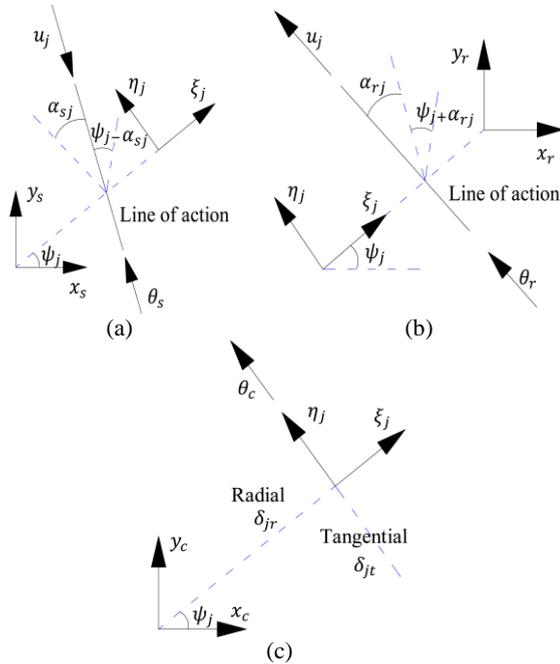
Fig. 3 Kinematics sketches to derive relative deflection components.
