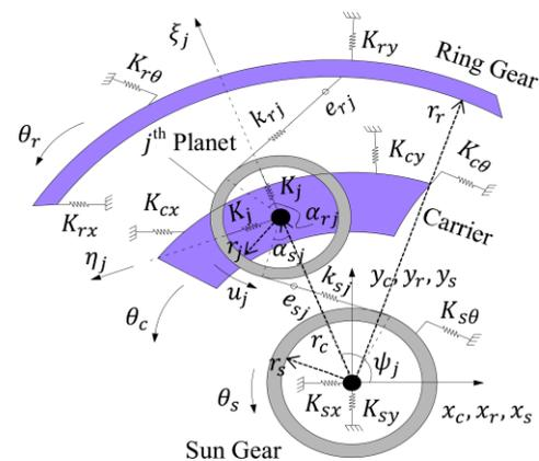
Fig. 2 Mesh of sun, ring and  $j^{\text{th}}$  planet bearings.
