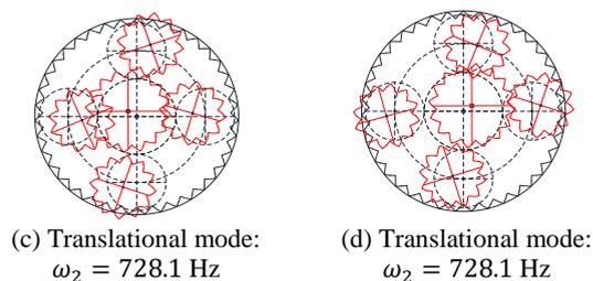
Fig. 13 Types of vibration modes of the SS with four planets (0, 90, 180 and 270 degrees).
