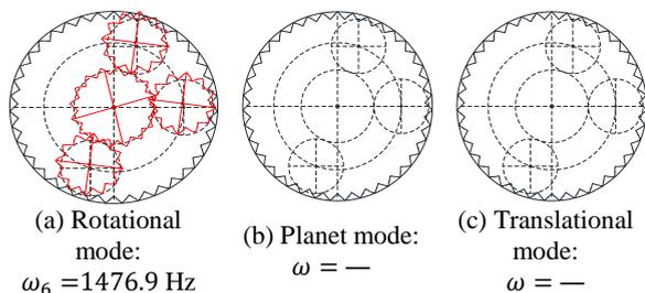
Fig. 10 Types of vibration modes of the ASS with three planets (0, 80 and 260 degrees).
