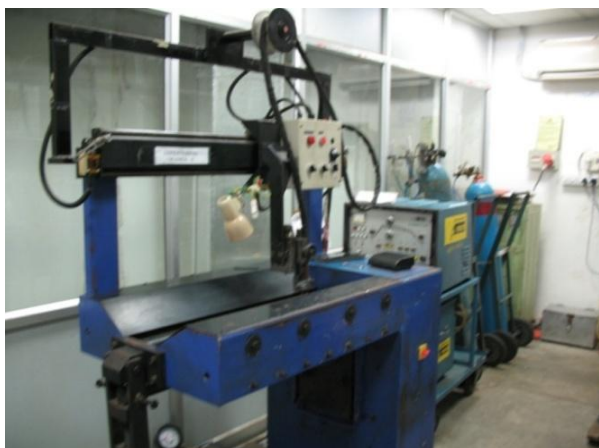
Fig. 1 Micro Plasma Arc Welding Setup.
